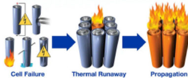
Figure 1: Diagram depicting a cascading thermal runaway event.
